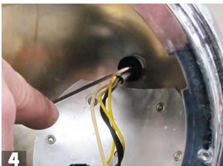
**4** Poke a 1/8"-diameter metal rod (clothes hanger) through the grommet in the housing to open it up and make room for the wire you need to thread through it next. Coating the rod with a little dielectric grease will help.
