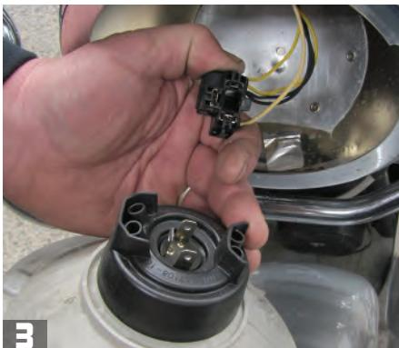
**3** Disconnect the headlight harness from the back of the stock headlight. (The headlight will not be reused.) If you don't want to connect the daytime running lights, jump to step 14.
