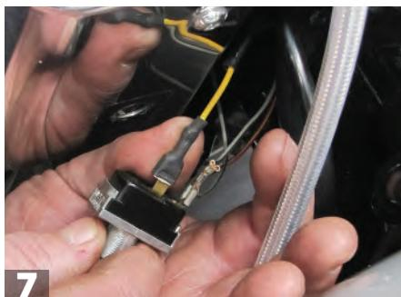
**7** Pull the yellow wire (the one that's activated when this switch is turned on) from the back of the switch.
