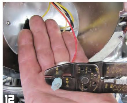
**12** Cut the wire you installed so about 7" of it is in the headlight bucket and bare about 3/8" of the wire. Then install a female blade connector on the wire and a male connector onto the short red wire on the new LED headlight plug.
