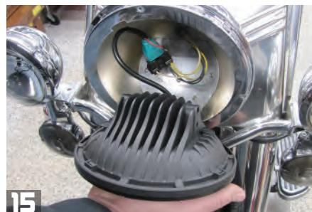
**15** Align the three tabs on the back of the new Cyron headlight to the three notches in the stock headlight bucket.
