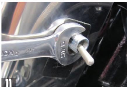
**11** With the switch properly orientated in the cover, secure the switch using the stock nut and a 9/16" wrench. Then thread on the circular nut to lock it in place. Tighten it with the pliers.
