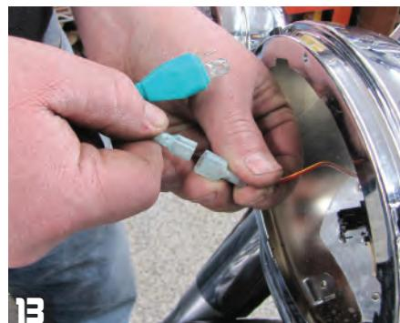
**13** Join the two connectors you just installed. Some people like to then wrap some electric tape over the two connectors.
