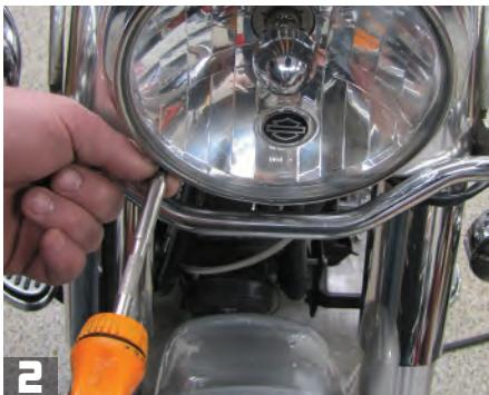
**2** Then remove the three screws that hold the beauty ring to the headlight bucket using a #2 Phillips screwdriver. Set this ring and these screws aside for reinstallation later on.
