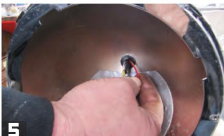
**5** Now poke an 18" length of 16-gauge wire through the rubber grommet and route it out of the left side of the triple tree covers.
