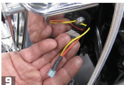
**9** After twisting the two wires together, slip a 1" length of heat shrink over the wires. With a crimping tool, put a new blade connector onto the wires and then use a heat gun to shrink the tubing.
