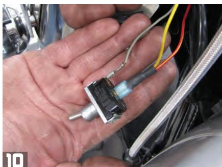
**10** Plug the new connector onto the back of the switch. Make sure it's secure. Then reinstall the switch in the left triple tree cover.
