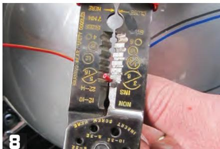
**8** Using wire strippers, bare about 3/8" of the 16-gauge wire you just ran. Also use wire cutters to remove the blade connector from the stock wire you just pulled from the spotlight switch and bare about 3/8" of that wire.
