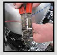
6. After twisting the two wires together, slip a 1" length of heat shrink over the wires. Then use a crimping tool to put a new blade connector onto the wires. Use a heat gun to shrink the tubing so you get a final result like this.
