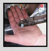
9. Cut the wire you installed so about 7" of it is in the headlight bucket and bare about 3/8" of wire. Then install a female blade connector on the wire and a male connector onto the short red wire on the new LED headlight plug.
