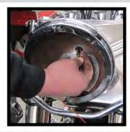
2. Now thread an 18" length of 16-gauge wire though the grommet and out of the left side of the triple tree covers.
