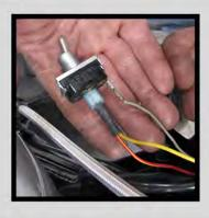
7. Plug the new connector onto the back of the switch. Make sure it is secure. Then reinstall the switch in the left triple tree cover.
